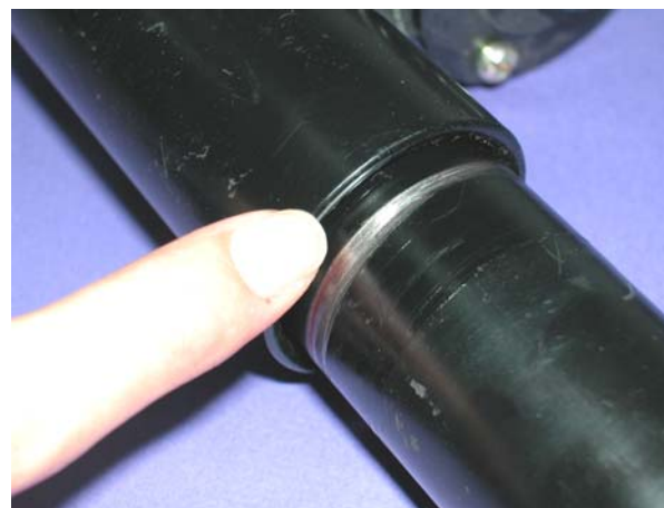
Step 2. Turn the incline motor pipe until the red line on the thin pipe is visible just above the end of the thick pipe.
