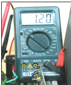
Step 3. Turn the VR gear until the multimeter shows 1.20 VDC.
